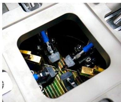
Typical MPI configuration with Kelvin Probes
