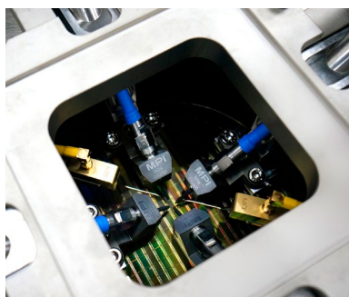
Typical MPI configuration with Kelvin Probes
